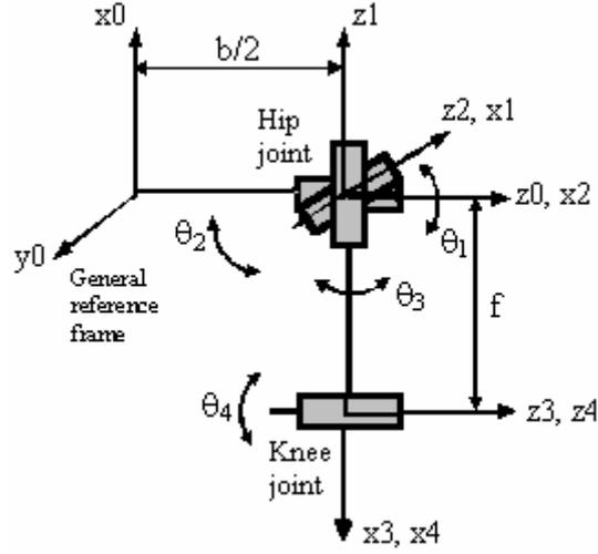
**Fig. 1.** Kinematics femur model
