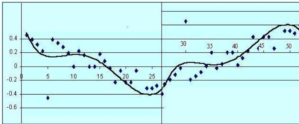
**Fig.3** Lower extremity femur motion during a half walking pace
